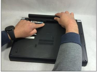
Slide the battery release slider all the way to the right and push the battery straight out of the back of the computer
