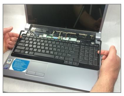
Starting at the top where you just removed the black panel, pry the black bezel away from the outside of the keyboard
