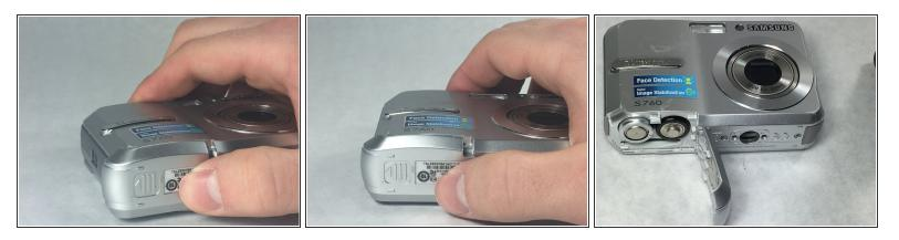
• Placing your thumb on the battery cover, push outwards, away from the camera in the direction the arrow is pointing. If done correctly when it's completely unhooked, the latch will open.
