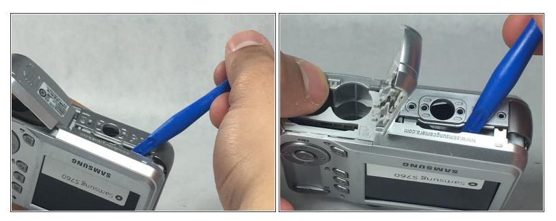
Use the plastic opening tool to pry open the back case, following alongside the edge of the case if need be.
