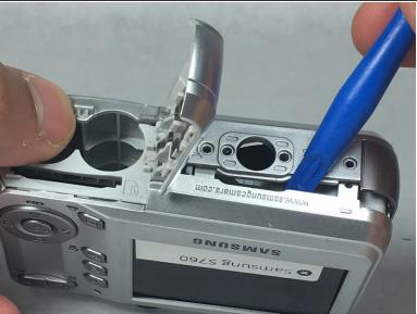
Use the plastic opening tool to pry open the back case, following alongside the edge of the case if need be.
