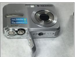
• Placing your thumb on the battery cover, push outwards, away from the camera in the direction the arrow is pointing. If done correctly when it's completely unhooked, the latch will open.
