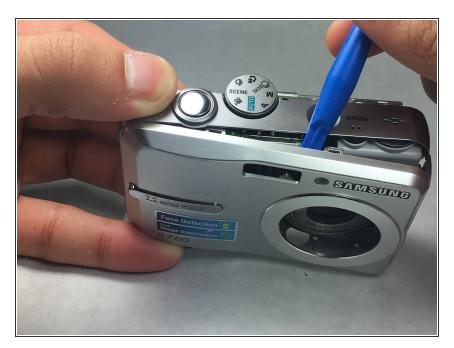
Once the back case is removed, use the plastic opening tool to gently pry off the front case.
