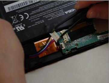
• Using needle-nose <u>tweezers</u>, gently push the large white wire connector (connected to the black, red and blue wires) out of its housing.
