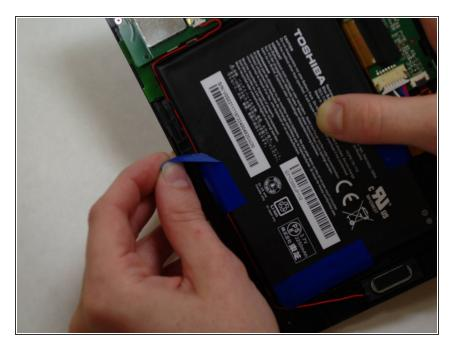
Carefully remove the electrical tape that holds the battery in place.
