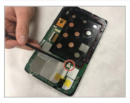
Use the spudger to pull the speaker wire plug from its socket.
