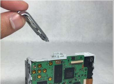
Pull the battery cover in the same direction you pushed to open it. The cover should come right off.
