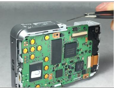
Using the tweezers, grasp and pull the portion of the pin that is sticking out of the hinge.
