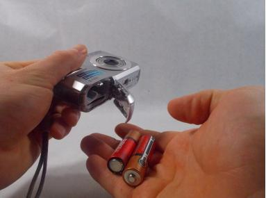
• Tip the camera as to gently slide the batteries out of the camera.
