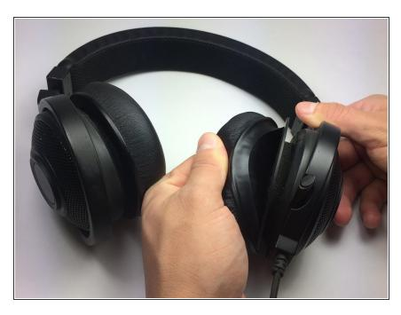
Pull the ear cushion away from the speaker by sliding down to release the cushion from the plastic covering.
