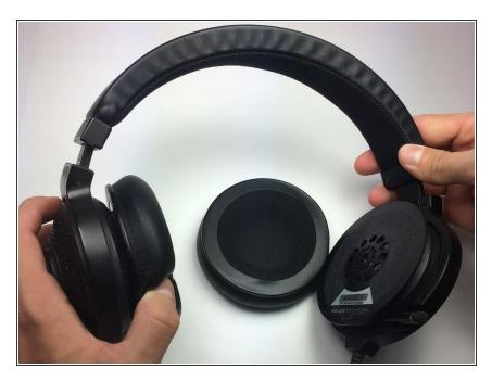
Continue sliding downwards around all edges of the ear cushion until the cushion is fully removed.
