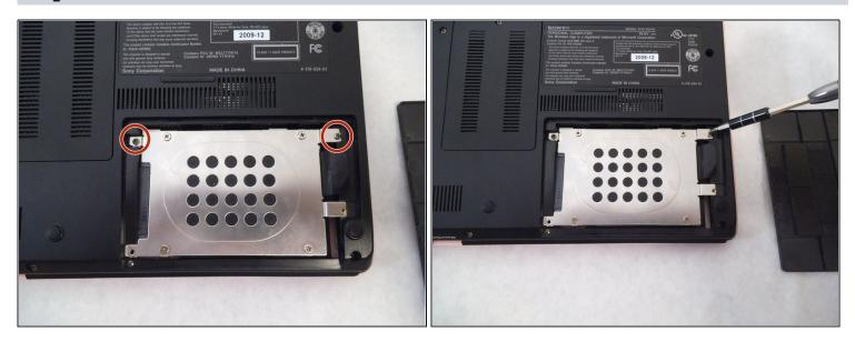
• Remove the two 4.8mm screws that are holding the hard drive down.
