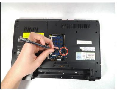
Remove the three 5mm screws that are holding in the keyboard.
