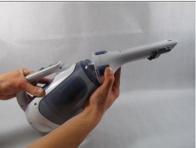
Disconnect the vacuum's nozzle by pressing the blue buttons on the side of the nozzle.
