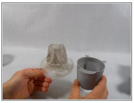
With the filter unit in your hand give the dark grey plastic shroud a quarter clockwise turn and remove the shroud exposing the filter.
