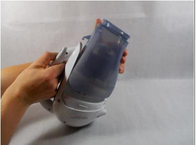
Disconnect the dustbin from the rest of the vacuum by pressing the blue button on the vacuum's handle.
