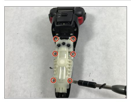
Using the Phillips 00 driver bit, remove six screws (12mm) from the battery case.
