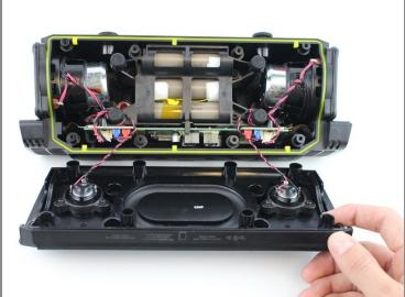
• Carefully untangle the wires that connect the speaker to the motherboard.
