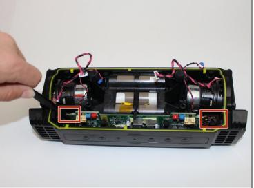
• Use <u>tweezers</u> to remove the two ribbon wires on the left and right side of motherboard.
