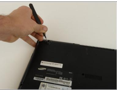
• Remove the top two rubber stoppers by grasping them with the precision tweezers and pulling up.
