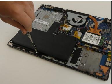
Remove the four 3 mm screws using the Phillips #000 screwdriver.
