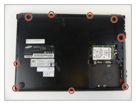
Remove nine 6mm cover screws using the Phillips #000 screwdriver.
