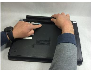
Slide the battery release slider all the way to the right and push the battery straight out of the back of the computer
