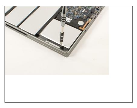
Remove the screws holding the battery in place.
