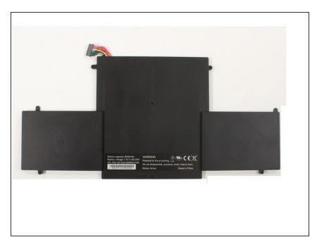
Make sure that the wattage and voltage matches the values of the old battery
