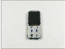
Once screws are removed, separate the motherboard and outer lens by carefully pushing the motherboard out with your hand as displayed in the image.
