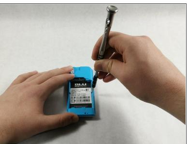
Using the phillips head screwdriver, remove all 5 2.5mm screws.
