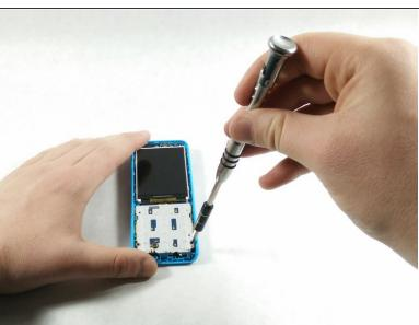
Locate the two 2.5mm screws (red circles in image) and remove them with the Philips 00 screwdriver used previously.
