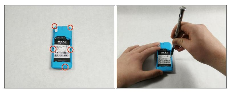
Using the phillips head screwdriver, remove all 5 2.5mm screws.
