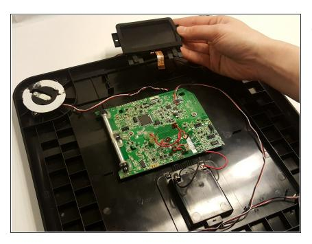
The screen should be free from all constraints and all that is left is to carefully lift and remove the screen.
