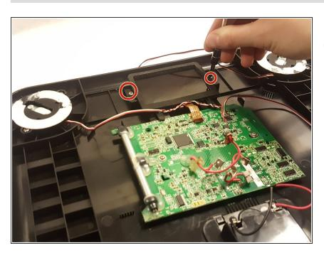
Using the Phillips screwdriver head, unscrew the two screws that hold the screen in place.
