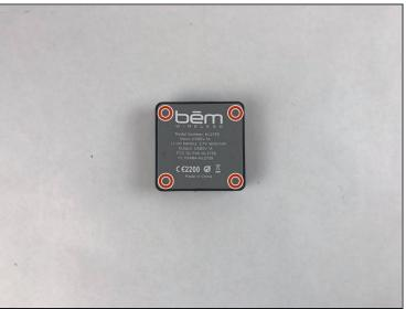
• Use the J1 bit attached to the screwdriver to remove the four 10mm screws from the bottom of the auxiliary charging base.
