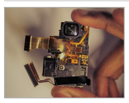
Using the tweezers carefully remove the broken/damaged lens with its attached circuit board
