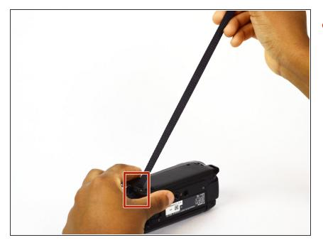
• Pull the strap through the slot on the left side of the camcorder.
