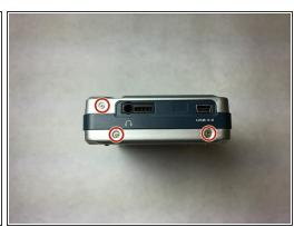
Use a J0 screwdriver to remove the eight 3.5mm screws.
