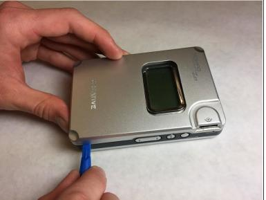
• Use plastic opening tool to open top cover by carefully prying at each corner.
