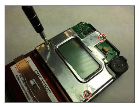
Once the front face is removed, remove the three 6.8mm J0 screws from the metal cover.
