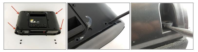
Use a plastic spudger to remove the rubber grommets from the four corners of the speaker underneath the mesh frame.
