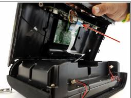
Separate the mesh frame and plastic frame by placing the spudger in between them.
