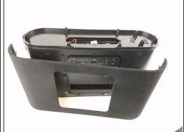
Pry off the mesh frame from the back side of the speaker with a plastic spudger until you hear a click noise when the clip is removed.
