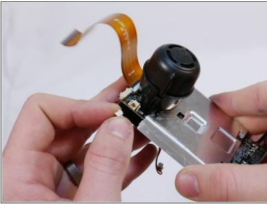
Find the power connector next to the buzzer that is labelled "MIC IR-LED". Use your fingers to wiggle it back and forth until it becomes loose.
