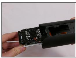
Grip the circular part of the motherboard and pull it straight out of the device.
