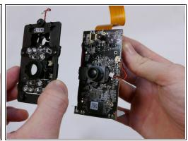
Lift the infrared LED board directly upwards and pull away from the motherboard.
