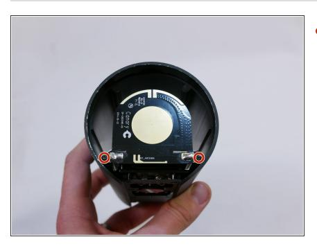
Use your Phillips #0 screwdriver to remove the two 5mm screws.
