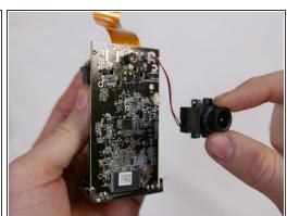
• Using your forefinger and thumb, grip the top and bottom of the lens assembly and pull away from the motherboard.
