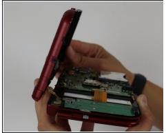
To separate the cover, carefully lift it up and away from the hinges (in order to clear the headphone port), then pivot it towards the hinges to expose the circuit boards.
