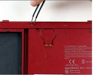
Using tweezers, carefully pop out the rubber bumpers located at the top side of the 3DS.
