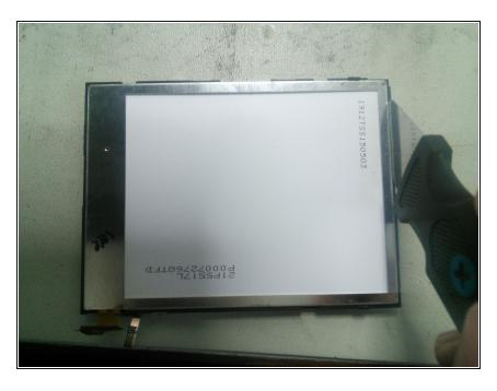
Slide a thin pry tool between the LCD and the black casing of the whole display, then lift it gently. The LCD comes out without forcing it.
