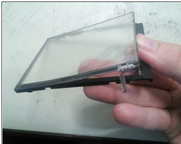
• Warm the edges of the touchscreen to peel it off more easily, then push it gently from underneath with your fingers to remove it.
