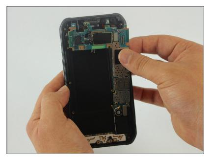
• Remove the motherboard from the rear case.
