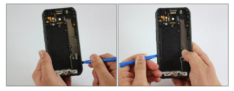
• Once you see a large enough gap, insert a plastic tool between the frame and the plastic cover and slide it around the phone to separate both components.
