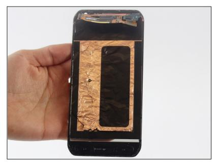
• Remove the display assembly (LCD and Digitizer).
