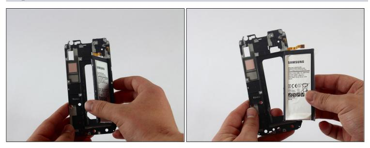
• Remove the battery from the frame.
