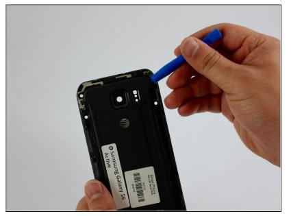
• Insert a plastic tool between the frame of the phone and the back cover at the top right corner.
