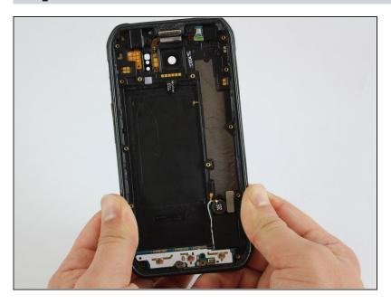
• Put a little pressure on the top, on the bottom, and on the sides of the phone to separate it from the plastic cover.
