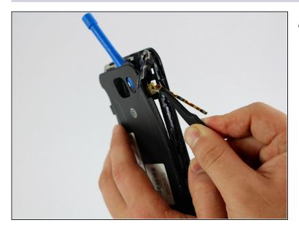
• Insert the <u>tweezers</u> under the contact points to undo the connection.
