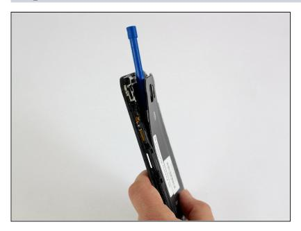
• Leave the plastic tool inside in order to access the volume button connection.
