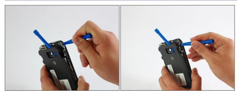
• Insert a plastic tool to pry open the black and beige piece covering the volume button connection.
