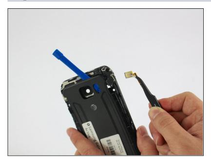
• Use the tweezers to remove the volume buttons bracket.
