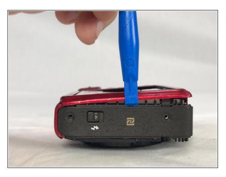
Use a plastic opening tool to loosen and remove both the front and back plates of the camera, as well as the two side pieces.
