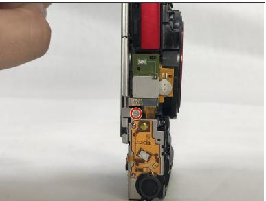
Unscrew the 2mm screw connections of the main board protector from the camera frame using a #000 Phillips head screwdriver (2 on front, 1 on top)
