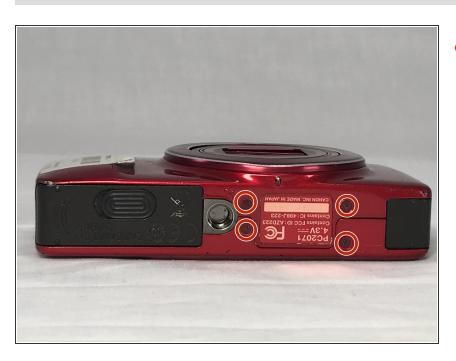
Unscrew the four 2mm located on the bottom of the camera using a Phillips #000 screwdriver.
