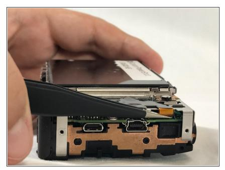
Use a pair of tweezers to remove the no-fuss connector from its holder.
