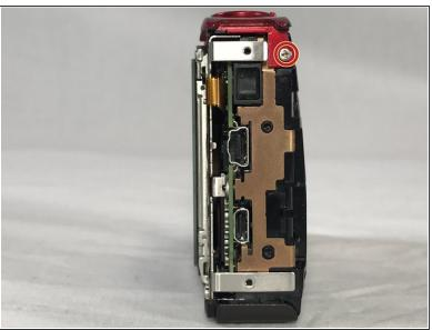
Unscrew the three 2mm screws attaching the piece to the camera frame with a #000 Phillips screwdriver.
