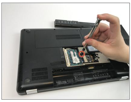
Inside the RAM panel, use the screwdriver to remove the 5mm screw pictured.
