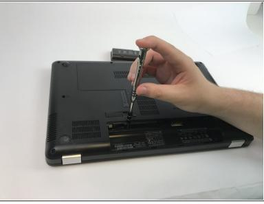
From left to right, unscrew the 5.5mm screw, the 7mm screw, and the 5.5mm screw located in the battery panel with the screwdriver.
