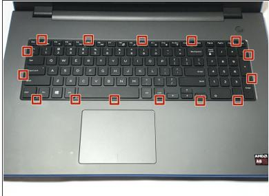
Open the display of the laptop as far as possible, and locate the tabs which secure the keyboard to the laptop.
