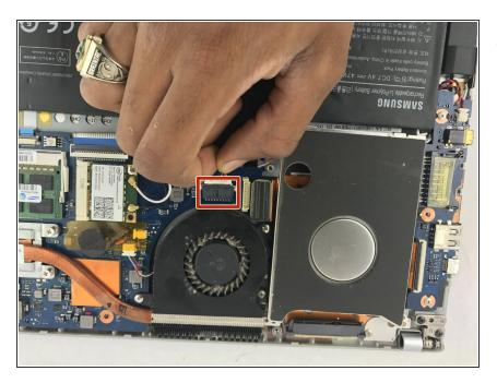
Now, detach the wire that is connected to the battery, which should now be removable.
