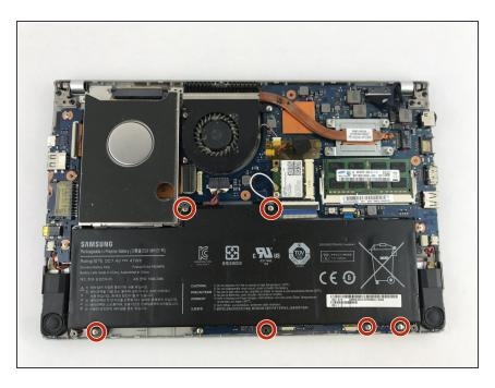
Now, locate the (4 mm) screws on the battery and remove them.
