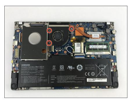
• Locate and unscrew the thre 4mm screws surrounding the fan.
