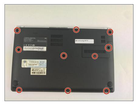
• First, remove the back of the laptop by unscrewing the (4 mm) screws shown using the PH0 screw bit.
