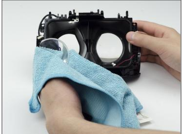
• Using a glass cloth (or any cloth with soft fibers), carefully press on the lenses until they pop out of place.
