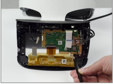
Using the <u>tweezers</u>, unplug the three (one black bundled, two multi colored bundled) connector cables from their ports along the circuit board.
