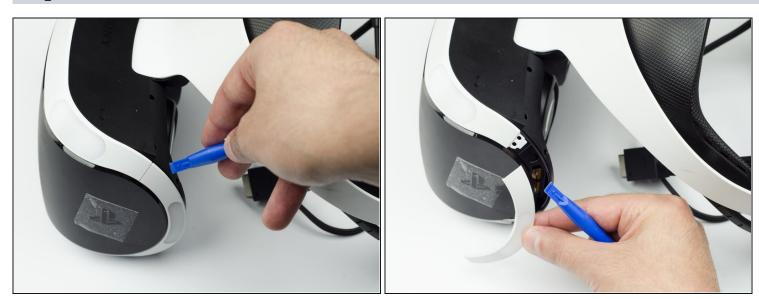
• Using the plastic opening tool, carefully pry the white plastic panel free from the side of the headset. Repeat this action for the opposite side.
