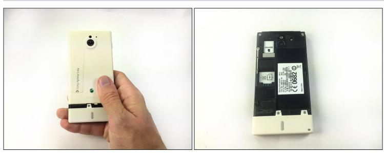
• Push the back cover as shown, then lift the cover off.
