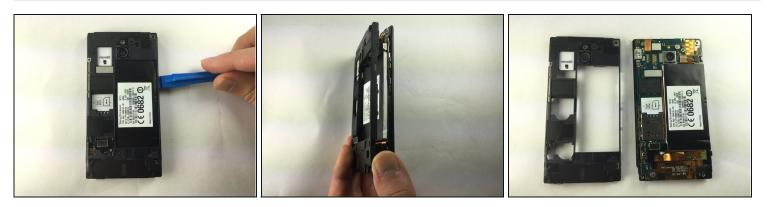
• Turn the phone onto its side and insert a flat object and gently remove cover, using plastic opening tool as shown.
