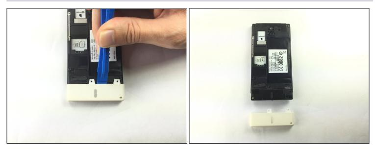
• Use plastic opening tool to remove the bottom white cover as shown.
