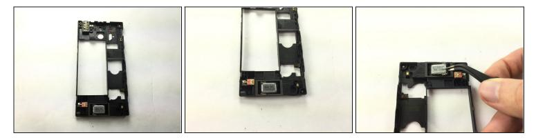
• Flip over the black back cover and locate the speaker phone at the bottom, then use the tweezers to remove the speaker. It is glued to the back cover so a little force will be needed.
