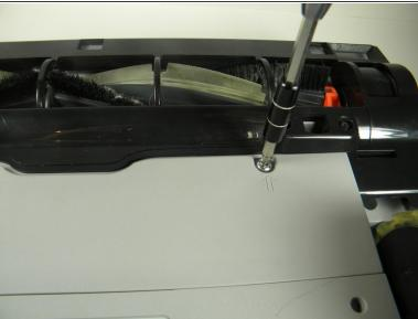
Use the Phillips #1 screwdriver to loosen both screws.
