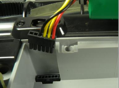
• Disconnect the current battery by pulling the connector from the base and pushing on the clip.
