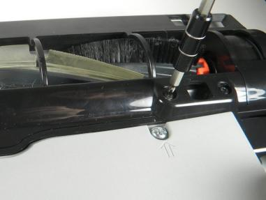
• Use the screwdriver to take off the four (4) 10mm screws located near the brush which secure the plastic guard.
