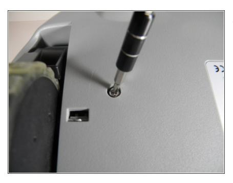
Remove eight (8) star screws using the T10 bit.
