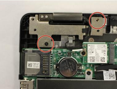
Unscrew the 7mm screws that secure the left and right hinges (using a ph1 screwdriver bit).
