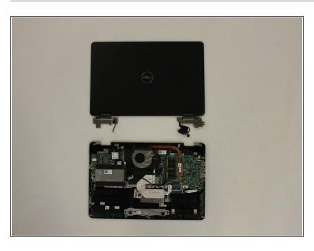
Carefully separate the screen from the bottom half of the device.
