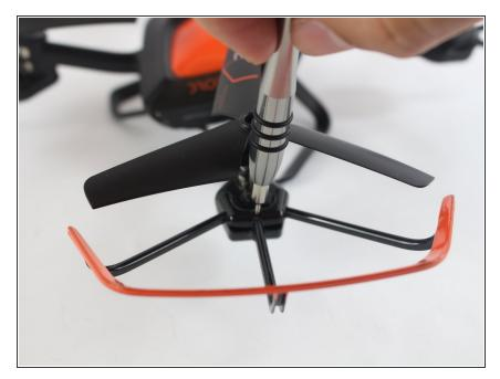
Remove the 9.1mm rotor guard screw found directly under the rotor blade using a Phillips 000 screwdriver.
