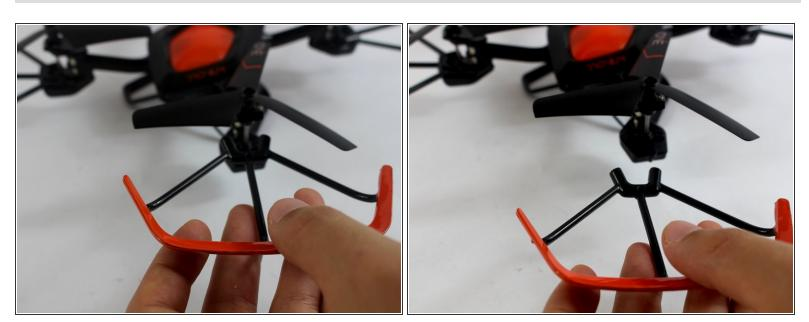
Carefully pull off rotor guard.
