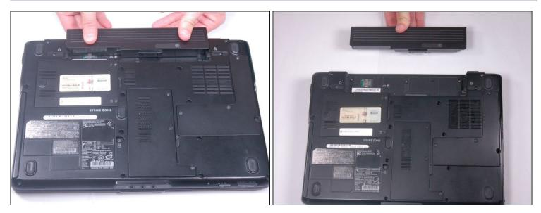
• Push the battery forward to eject it from the laptop.
