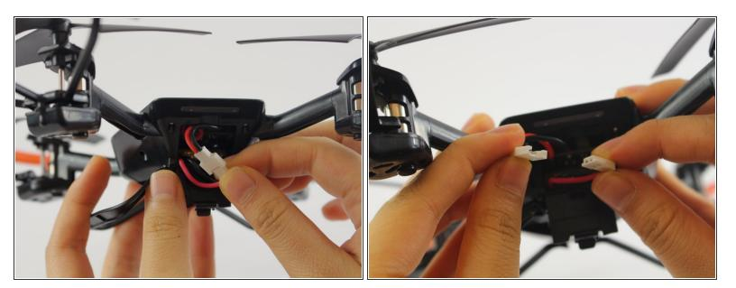
Expose the cable connection and pull apart the cable connection.
