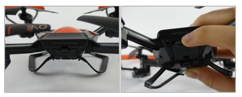
Pull down and out on the battery cover in the back of the drone.
