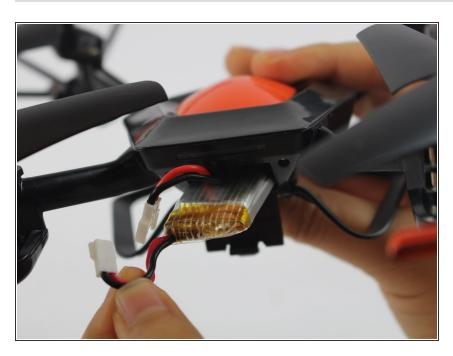
Carefully slide out the drone battery.
