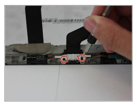
Using the PH000 screwdriver, remove the two black 3mm screws at the bottom of the device.
