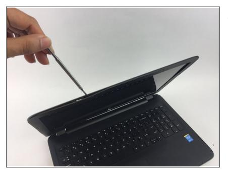
Use the black nylon spudger to separate the front frame and the back cover of the laptop. Start at the top and work your way around the screen.
