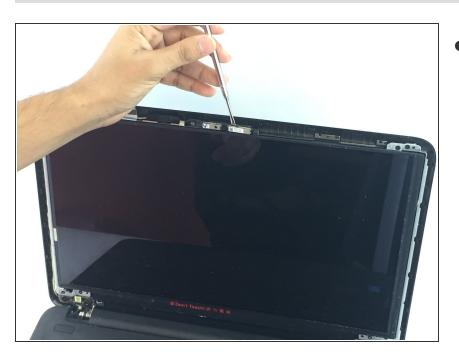
• Use spudger to separate the camera from the frame.
