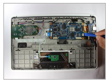
Using the plastic opening tool lift the motherboard out of the back panel.
