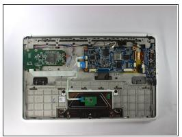
Remove the three 1.2mm screws using the Phillips #1 screwdriver.
