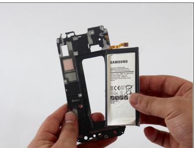
Remove the battery from the frame.
