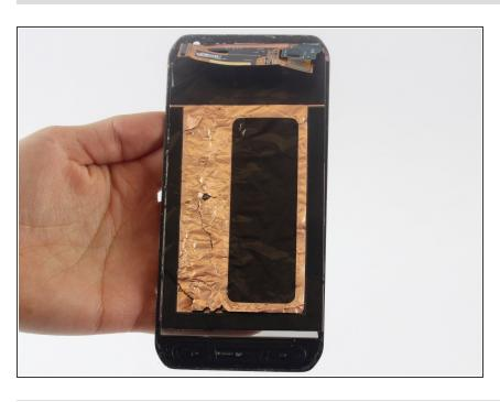
Remove the display assembly (LCD and Digitizer).
