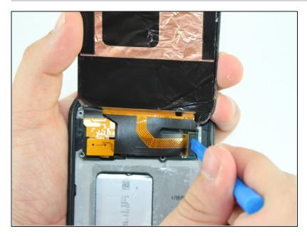
• Undo the screen connection with a plastic tool.
