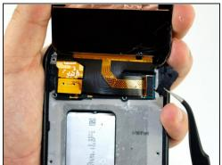
• Once the glass is off, you will see a small clip covering the screen connection to the motherboard at the top of the phone. Use <u>tweezers</u> to grab the clip by the crease on its side and pull it out.
