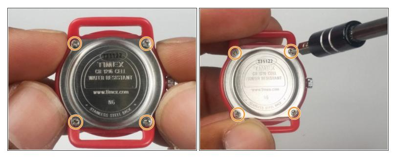
• Use the PH00 screwdriver to remove the four screws from each corner of the rear metal cover.
