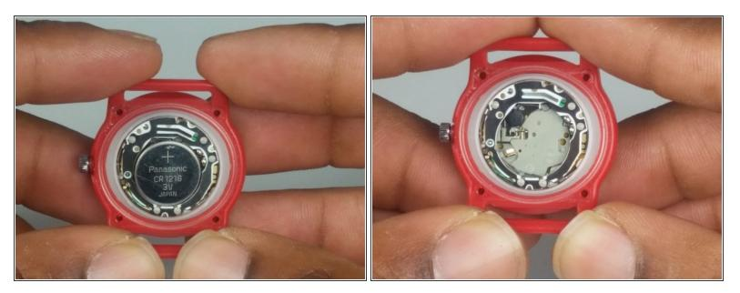
• The battery spring will propel the battery upward as soon as the base cover is removed. Be sure to place the battery in a safe spot.
