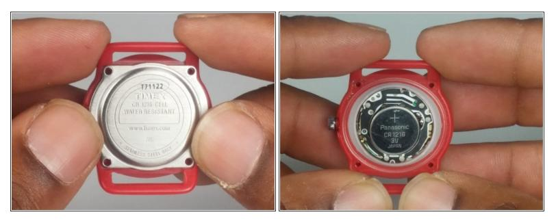
• Gently remove the back plate to expose the battery.
