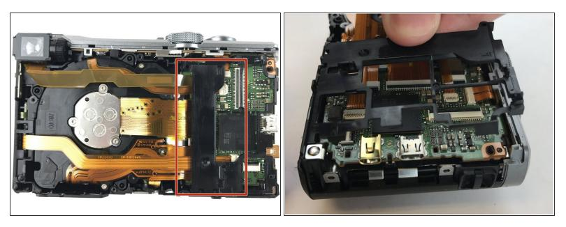
Pry the black cover shielding the ZIF connectors off with your hand.
