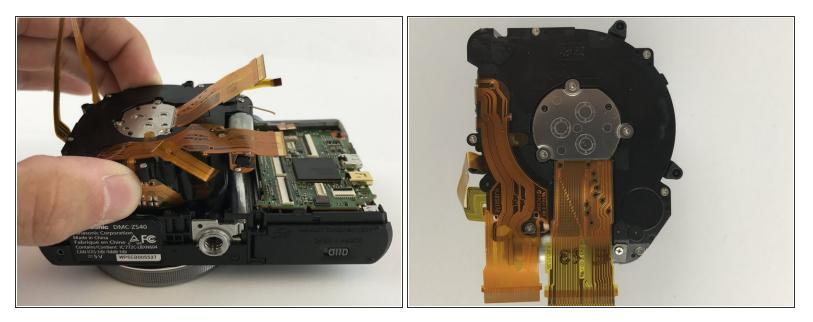
Once the corresponding ribbon cables have been detached, the lens assembly can be lifted right up.
