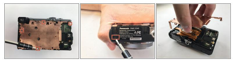
• Remove these four 4mm on the top of the plate cover and the 3mm screw on the side of the camera using a PH000 bit head. Once the screws are removed, the plate cover should lift right up.
