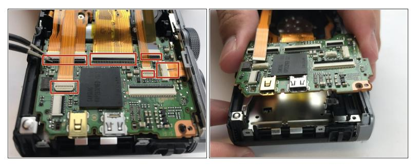
Disconnect these 6 ribbon cables from the motherboard. Use tweezers or a screw driver to lift up on the retaining flaps for each ZIF connector.
