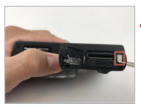
Push up on the right-hand-side tab to release the battery.
