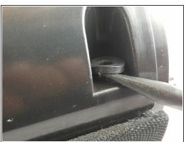
• Use a plastic spudger to remove the rubber grommets from the four corners of the speaker underneath the mesh frame.
