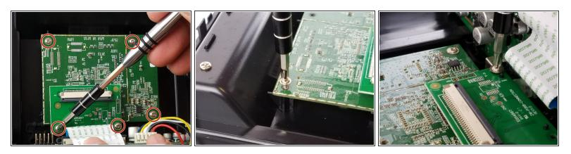
Unscrew the five 11 mm Philips #1 screws found on the outside of the circuit board.
