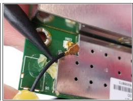
Pry the glue and unclip the wifi antenna plug from the circuit board.
