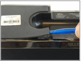
Remove the rubber from the bottom of the speaker, use a medium blue plastic spudger to gently
