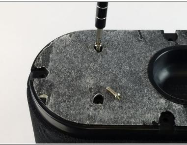
• Remove the two remaining 11 mm Philips #1 screws holding the base and set them aside.
