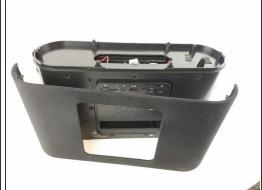
Pry off the mesh frame from the back side of the speaker with a plastic spudger until you hear a click noise when the clip is removed.
