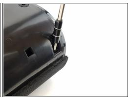
Remove the four 11 mm Philips #1 screws from beneath the rubber grommet that was removed from the previous step in all four corners.
