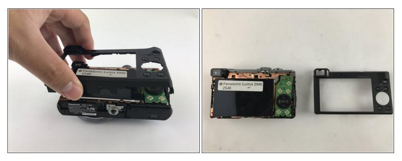
• Pry off the back casing of the camera and place the camera face down.
