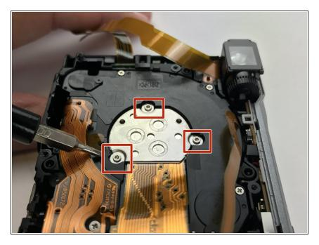
• Using the T3 Phillips Screwdriver, unscrew the three Torx T3 2.5mm screws holding the sensor down.
