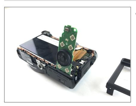
• Flip the right hand side control dial circuit board up.
