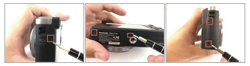
Unscrew these five 3mm screws located around the sides of the camera using a screw driver with a PH000 bit head.
