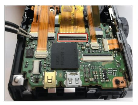
Remove the ribbon cable connecting the sensor to the motherboard. Use tweezers or a screw driver to lift up on the retaining flap of the ZIF connector to remove the cable.
