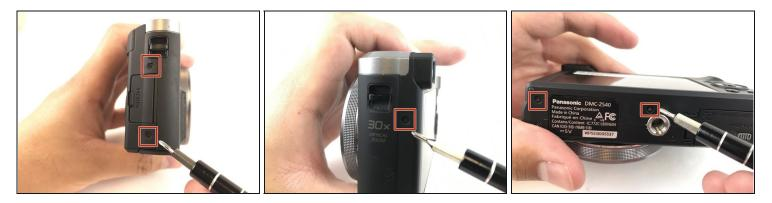
• Unscrew the five 3mm screws located around the sides of the camera using a PH000 bit or Phillips 000 Screwdriver.
